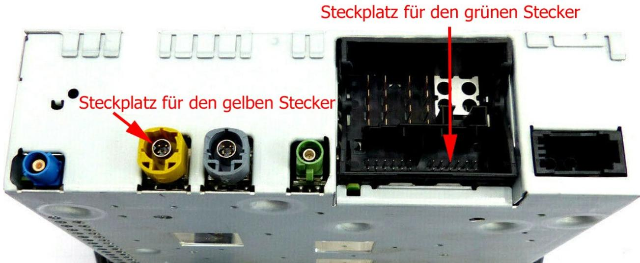
1. The unit is connected directly to the rear of the radio (A4/A5/Q5 in the centre console, A6/A8/Q7 in the glove compartment). The yellow plug is plugged into the yellow socket and the green plug is plugged into the main plug at the bottom right. If an AUX or AMI is already installed, please unplug the original connectors. AUX/AMI lose their function.
